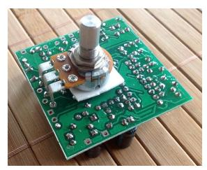
Next put the board mounted pot on the backside. Please cover the pots backside with tape so there cannot be any shortcuts with the solder pins of the populated board. Don't forget to clip off the notch.
