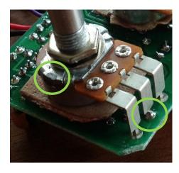
The board mounted pots need to go onto the other side of the board. Use some (double-sided) tape to make sure the pot cases do not shorten any pins that come through the board. As you solder them it is good practice to apply some solder to the middle pin first, then pull it back or approx. 1mm and let it harden. Then solder the other pins. This will align the pot horizontally in a better way and avoid shortcuts of the wide pot pins and the board.
