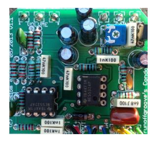
If you are unable to source 3n9 capacitors. Use a Mylar 2n7 and a ceramic 1.2 in parallel (yes, they fit through one hole) and you are there.
