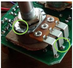
The board mounted pots need to go onto the other side of the board. Use some (double-sided) tape to make sure the pot cases do not shorten any pins that come through the board. As you solder them it is good practice to apply some solder to the middle pin first, then pull it back approx. 1mm and let it harden. Then solder the other pins. This will align the pot horizontally in a better way and avoid shortcuts of the wide pot pins and the board.
