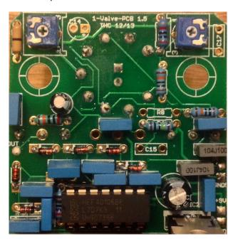
Start populating the small diodes first, then larger diodes, resistors, IC socket and capacitors. Then mount the 3mm LED from the backside. Make sure it is the right orientation before you solder the NOVAL socket on top of it. Of course this does only work if your tube socket has a hole in the middle. If not and it is a plastic socket, you can drill one. If its ceramic you will not get a hole in. Leave some space between tube socket and PCB!
