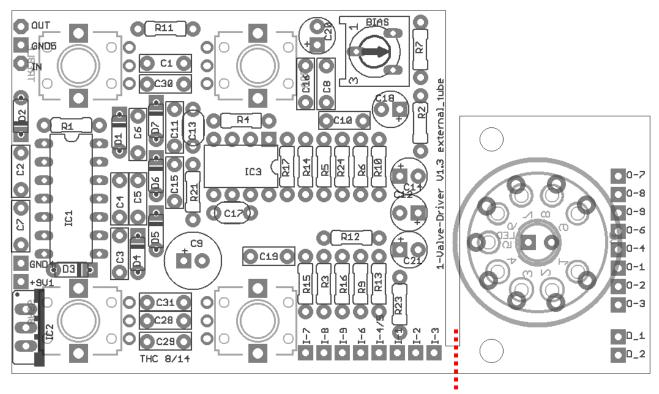
Start populating the small diodes first, then larger diodes, resistors, IC socket and capacitors. It is a good idea to mount the power regulator to the enclosure which will work as a heatsink.
