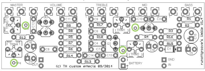
Make sure you wire the board before you mount the pots in as due to the small size of the board the wire holes will be hidden underneath the pots!
